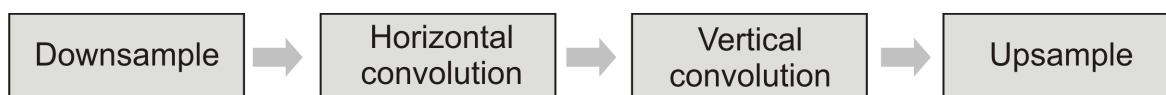
Figure 4-11: An optimization of Gaussian convolution proposed by Krawczyk et al. [KMS05], which allows full 8-scale local tone mapping at interactive frame rates. Each input texture is downsampled by a carefully selected factor, convoluted horizontally and vertically by a down-scaled approximation of the horizontal and vertical components of the Gaussian kernel, then upsampled back to its original dimensions.
